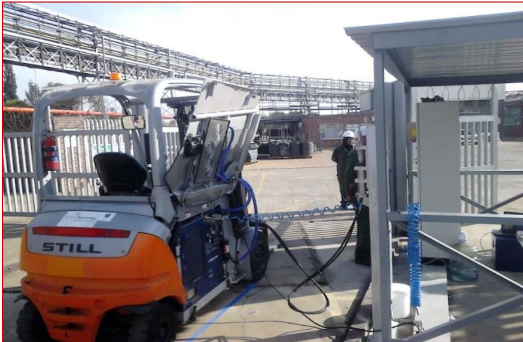
Hydrogen Fuel Cell powered forklift
