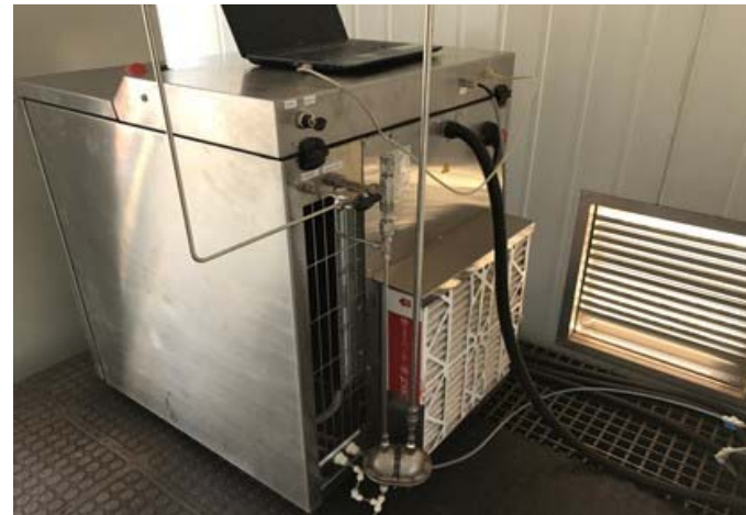
On-site hydrogen production and storage system
