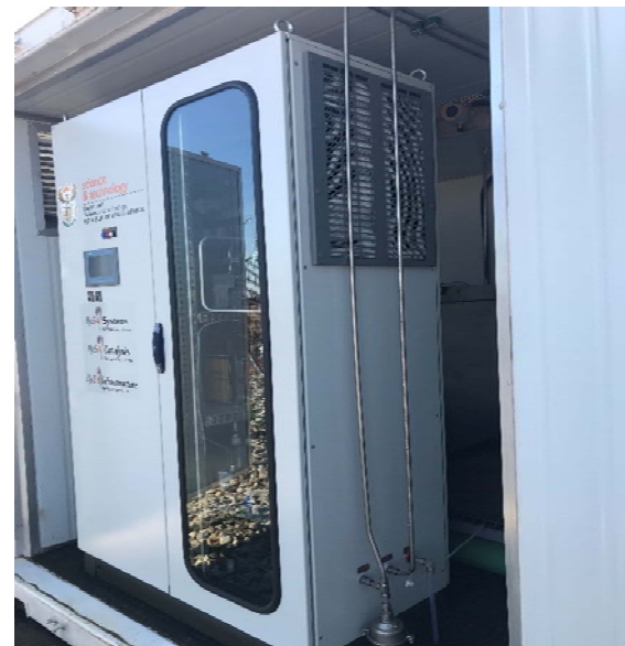
2.5 kW Hydrogen Fuel Cell System
